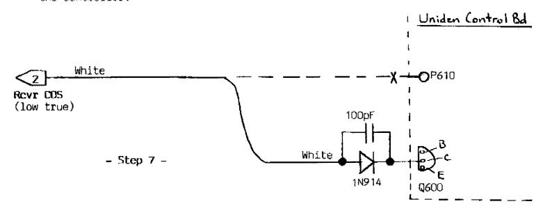
8. If CTCSS operation is desired, make the following modifications: Check the 9-pin Accessory Connector for a spare (unused) pin. If none is found, obtain a 0.062" Molex pin and connect it to a length of wire.
